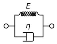
The Kelvin-Voigt model, also known as the Voigt model, consists of a Newtonian damper and Hookean elastic spring connected in parallel, as shown in the picture. It is used to explain the creep behaviour of polymers.
