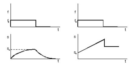
The response of Kelvin Voigt's and Maxwell's environments to the tension impulse (s=strain, t=time)
